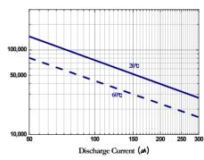
$\ensuremath{\mathscr{H}}$  This data was made on basis of nominal capacity for the purpose of enabling users to forecast approximate life time.
