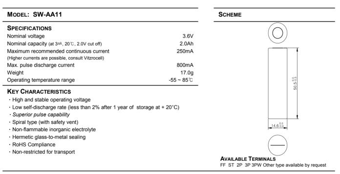
※ Max. pulse current/0.1 second pulses, drained every 2 min at + 20 ℃ from undischarged cells with 10 µA base current, yield voltage readings above 3.0V. The readings may vary according to the pulse characteristics, the temperature, and the cell's previous history.
