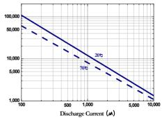
\* This data was made on basis of nominal capacity for the purpose of enabling users to forecast approximate life time.
