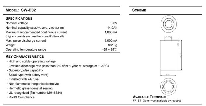
Max. pulse current/0.1 second pulses, drained every 2 min at + 20 °C from undischarged cells with 10 μA base current, yield voltage readings above 3.0V. The readings may vary according to the pulse characteristics, the temperature, and the cell's previous history.
